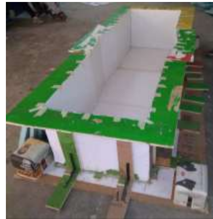
Fig -2: Final wooden pattern
