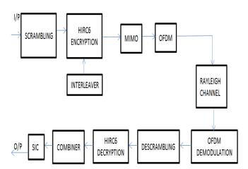
Figure 2: Block diagram of the system
