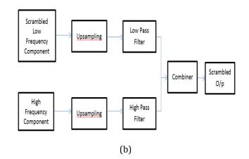
Figure: 1. (a) Scrambling based on morlet wavelet transform. (b) Reconstruction of the scrambled signal
