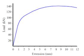
Figure 10. Load vs. displacement graphs for tensile test.
