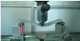
Figure 4. Flexural testing of the specimen.
