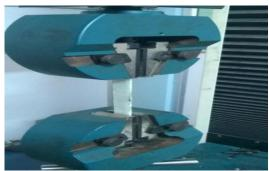
Figure 5. Tensile testing of the specimen.
