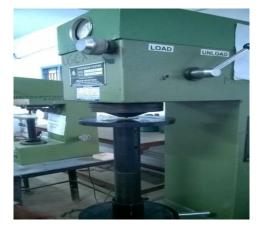
Figure 7. Hardness testing of the specimen
