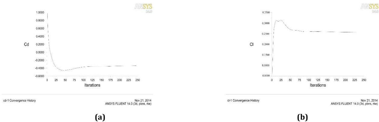
Fig 7: (a) Drag coefficient and (b) Lift Coefficient of base model car
