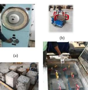
**Fig - 1**: Hydraulic CTM (a), Mold for accelerated curing (b), Spec (c) mmersed into warm wa curing (c) and accelerated cubes rea (d) accelerated strength test (d).
