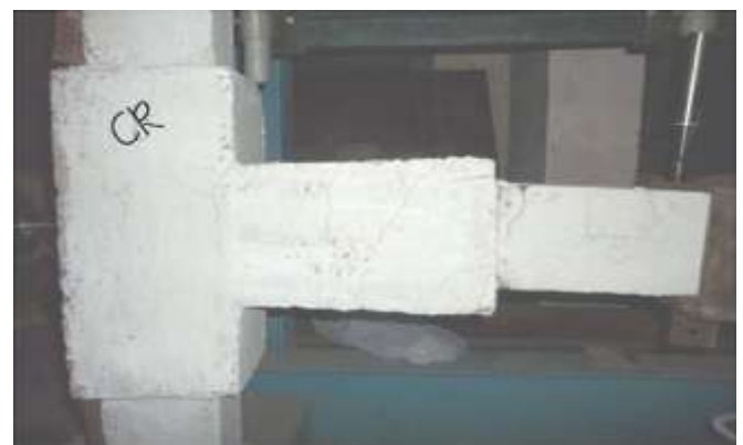
Fig-9: Failure pattern of conventionally retrofitted specimen
