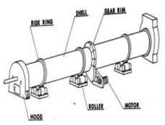
Fig.2 Construction of Calcination Drum.
