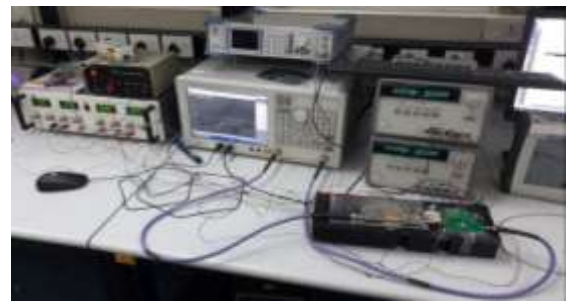
Figure.8. Experimental setup for testing the transmitter chain
