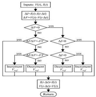
Fig -7: Flow chart of Incremental Conductance method.
