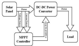
Fig -2: Block diagram of a MPPT controlled PV system.
