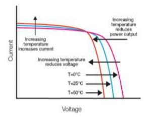
Fig -4: Power-voltage and current-voltage characteristics of a PV module for different cell's temperature at constant radiation level.
