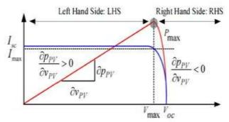
Fig -8: I-V and P-V curve and maximum power point of PV module.
