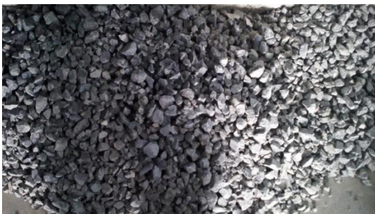
Fig No 2.2.3 Recycled Coarse Aggregate
