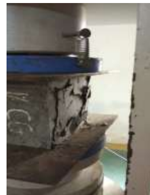
Fig-1: Interface transition zone failure
