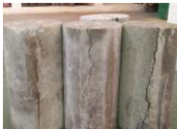
Fig-2: Cracks formed on cylinder after split tensile test
