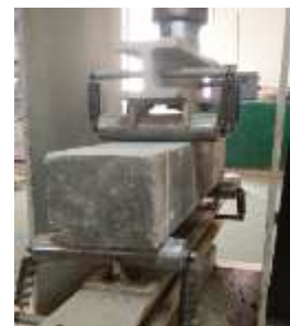
Fig-3: Application of three point loading on beam
