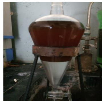
Fig -3: Water Wash of Biodiesel
