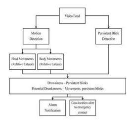
Fig. 2.1: Driving fitness detection- system flow diagram
