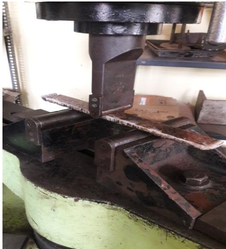
Fig-9: Specimen placed in Universal Testing Machine
