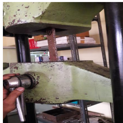
Fig-8: Specimen placed in Universal Testing Machine
