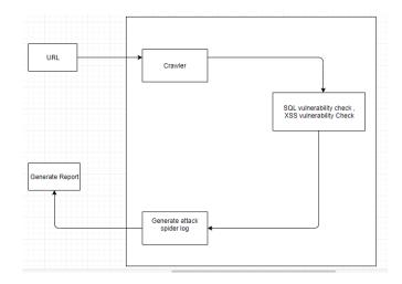
Fig.4.1 System Architecture diagram
