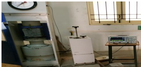
Fig 3- Experimental set up for a cube with embedded patches
