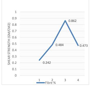
SHEAR STRENGTH OF FLY ASH WITH 12mm RECRON FIBRE WITH DIFFERENT LIME%
