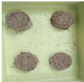
Fig -1: Arrangement of soil sample for the filter paper test
