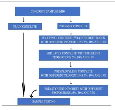
Compression test are done on 28<sup>th</sup> day of proper curing in fresh water.
