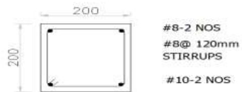
Fig -4: Detailing of plinth beam
