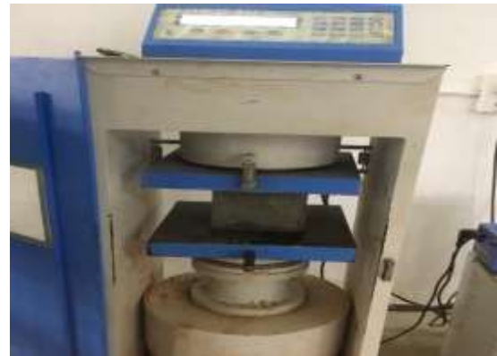
Fig -3: Compression test on cube
