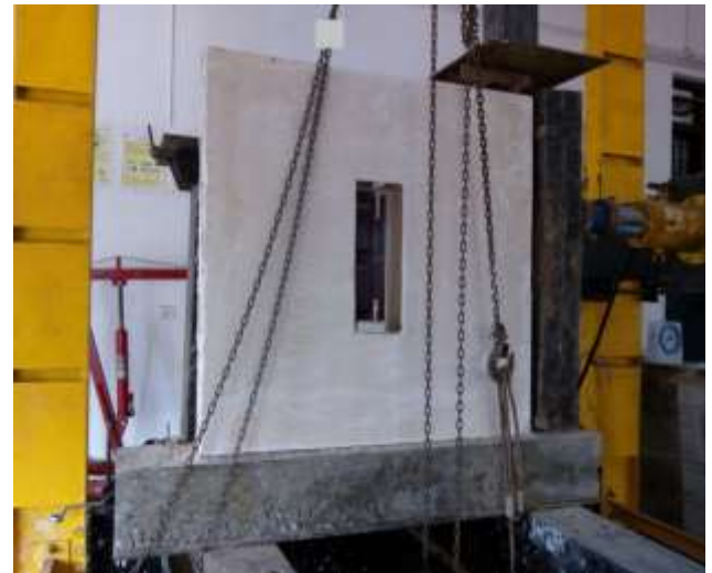
Fig-8: Testing of panel with opening
