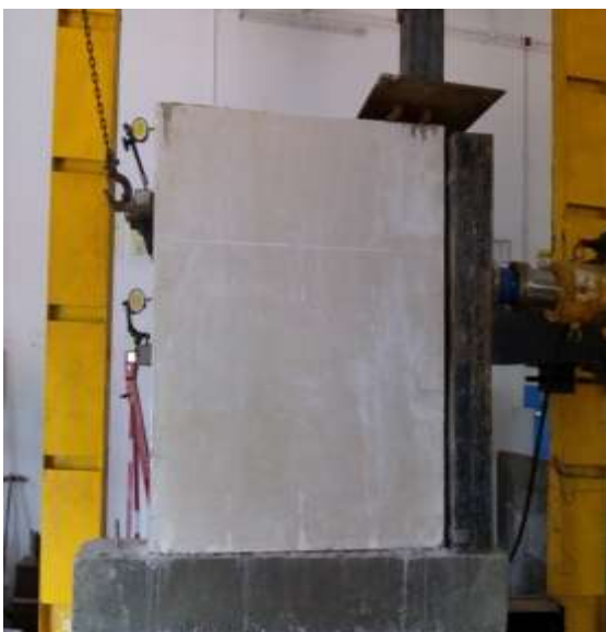
Fig-7: Testing of panel without opening
