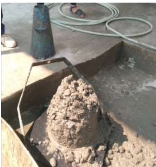
Fig-2: Slump obtained for M20 concrete
