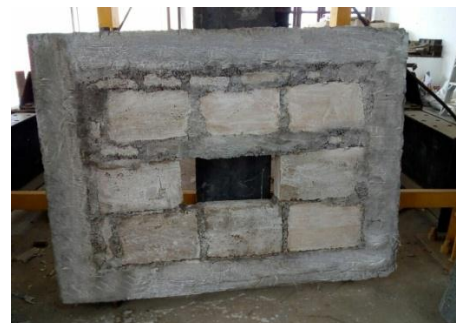
Fig- 2 Frame infilled with MCB with opening
