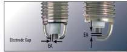
Fig.2 Spark gap of the Spark plug
