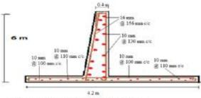
Figure 3.3.3 Reinforcement Detailing 1
