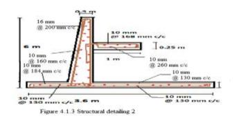
**3.3** Analysis and Design of cantilever Retaining wall with shelves : (Reducing its dimension up to maximum value)
