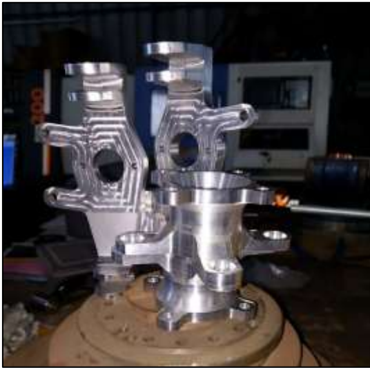
Fig -13: Manufactured Upright and Hub.
