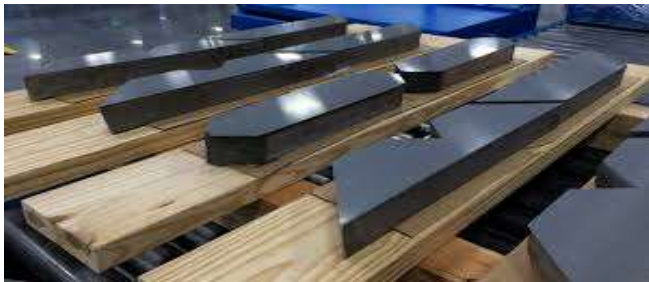
Fig -2: CRGO lamination
