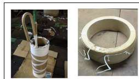
Fig -7: Coil Insulation
