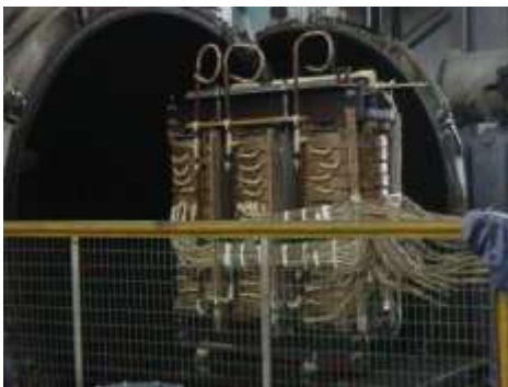
Fig -12 Core assembly in Oven
