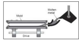
Fig -1: Schematic of horizontal centrifugal casting[2]
