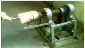
Fig -2: Horizontal centrifugal casting machine setup
