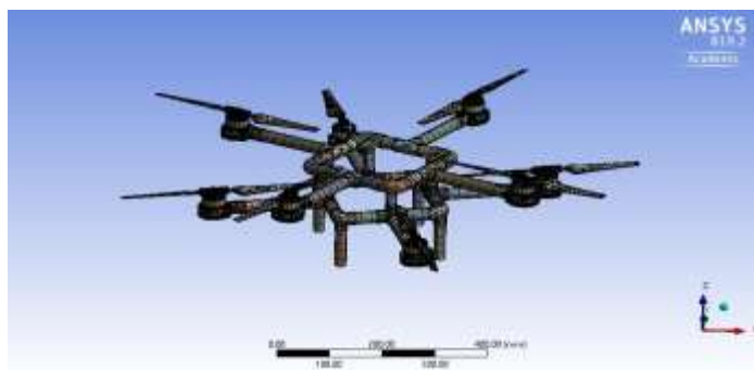
Fig -10: Meshing model of Octo copter drone
