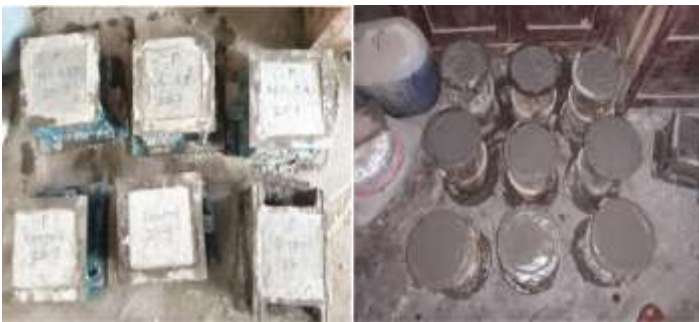
Fig 3.2 - Casting of Cubes & Cylinders
