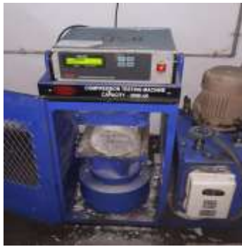
Fig 4.1- Compression Testing Machine using for Cylinders
