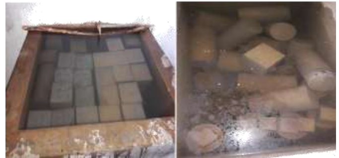
Fig. 3.4- Curing of Concrete
