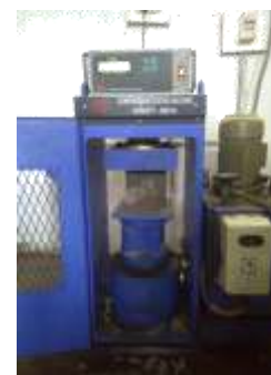
Fig 4.1- Compression Testing Machine using for Cubes
