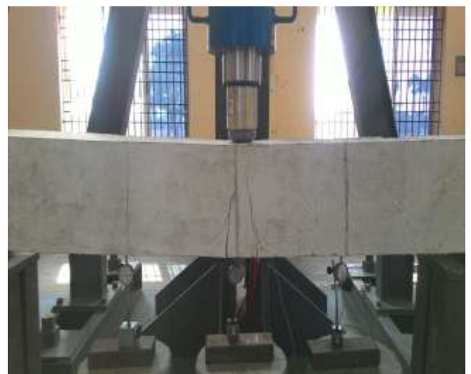
Fig -2: Flexural Strength Test
