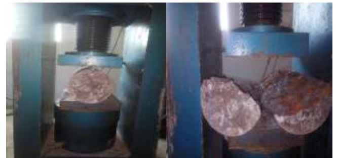
Fig-3 Cylinder Specimen Showing before and after failure
