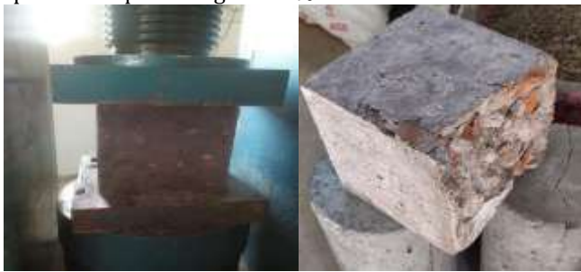
Fig-2 Cube Specimens Showing before and after failure
