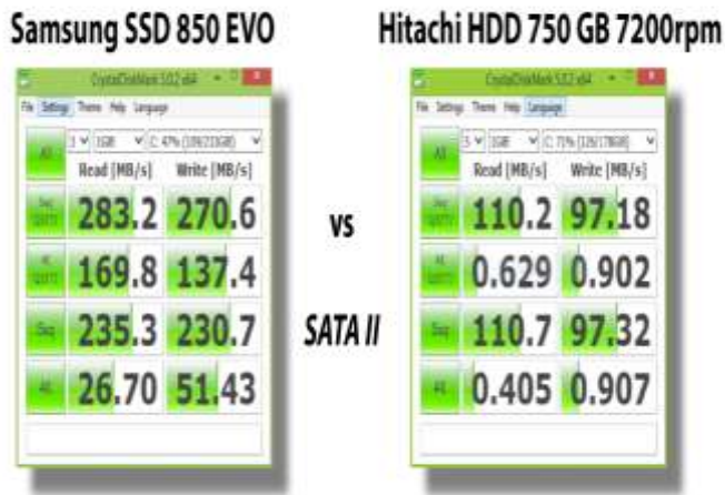
Fig 2.2 comparison Between SSD and HDD using For testing, Samsung SSD 850 EVO (SSD) and Hitachi HDD is used. From the test we can observe SSD having more read write speed.
