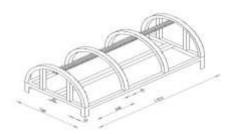
Fig. 1: Schematic diagram of solar tunnel dryer
