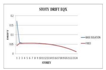
**Fig-6**: Comparison of story drift in fixed base and base isolated structure for load case EQX
