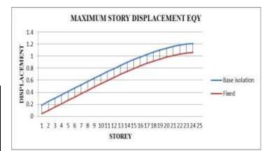
Fig-4: Comparison of story displacement in fixed base and base isolated structure for load case EQX
