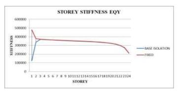
Fig-9: Comparison of story stiffness in fixed base and base isolated structure for load case EQY
