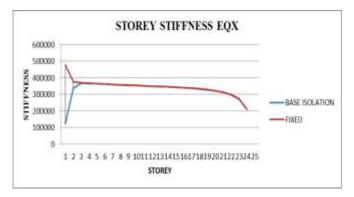
Fig-8: Comparison of story stiffness in fixed base and base isolated structure for load case EQX
