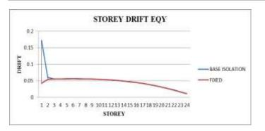
Fig-7: Comparison of story drift in fixed base and base isolated structure for load case EQY
