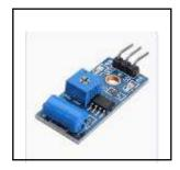
Fig-1: Vibration Sensor
