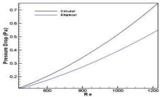
Fig -4: Variation of Pressure drop with Re
