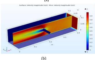
**Fig -3**: Velocity distribution for Re = 876
