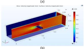
**Fig -2**: Velocity distribution for Re = 438
