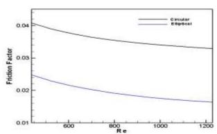
Fig -5: Variation of Friction factor with Re
