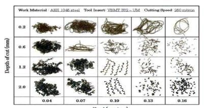
Feed (mm/rev) Chip chart in terms of feed and depth of cut.
