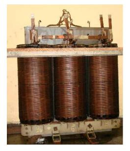
Fig. 1 Core assembly out of tank
