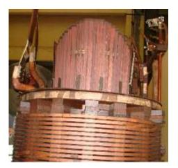
Fig. 2 one leg of Core assembly
