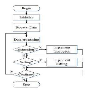
Fig-5 Flowchart of sink Node
