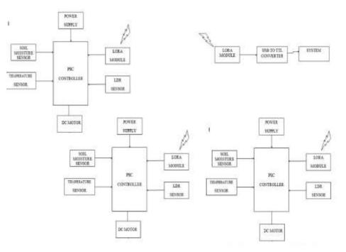
Fig-3 System Block Diagram
