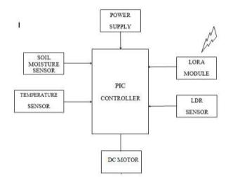
Fig-6. Block Diagram of Sensor Node.
