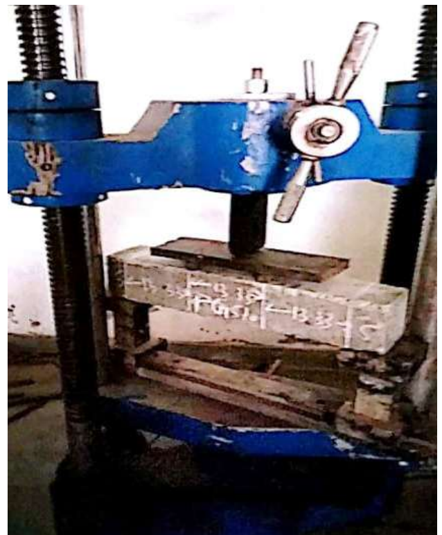
Beam placed in UTM during loading
