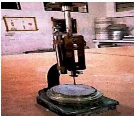
Vicat apparatus determination of final setting time
