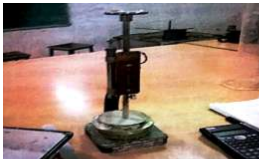
Vicat apparatus determination of initial setting time
