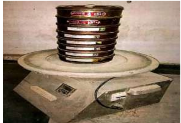
Sieve analysis of PG by using sieve shaker
