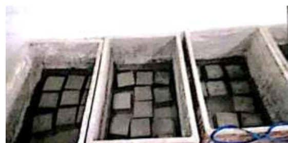
Curing tank containing cube sample
