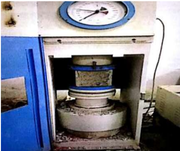
Cube placed in CTM during loading
