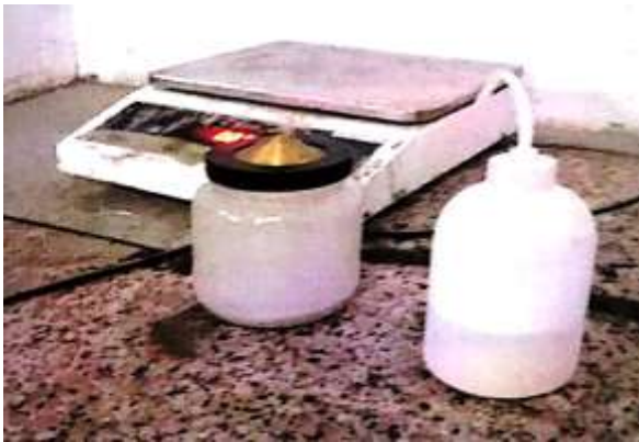
Specific gravity determination of PG sample by using Pycnometer
