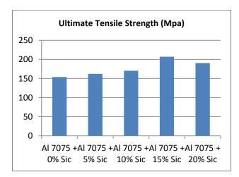
Fig: 7: Comparison of Ultimate Tensile strength
