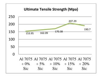
Fig: 8: Variation of Ultimate Tensile Strength
