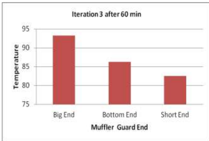
Graph-3-Temperature vs. Muffler Guard End for Iteration 3
