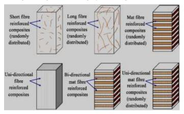
Fig -1 Different type of fiber orientation used for laminate manufacturing [18]
