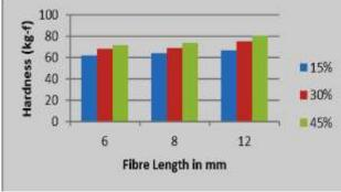
Fig -3: Effect of fiber parameters on Hardness of composites [35]
