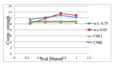
Fig. 3 Effect of soil content on 7days compr. Strength
