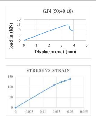
Fig-3. Stress v/s strain for tensile test
