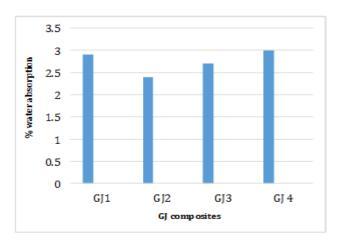
Fig-6. Water absorption tested Specimen
