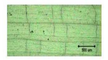
**1.4 Cracking Or Buckling**-Cracking or buckling takes place when a sandwiched composite is put under an excessive compressive load. When the load exceeds the limit of the structure, the core buckles and leaves a fracture line in the core which often takes the shape of a "smile" centered below the impact site.
