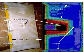
Fig 2. B747 outboard spoiler (left) and its resulting tap test image(right).
