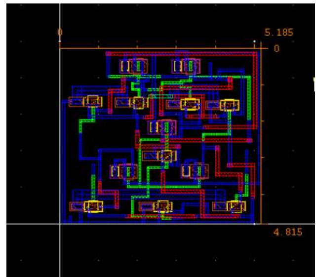
Fig -5: Layout design of the proposed comparator circuit schematic using cadence virtuoso 45nm tool
