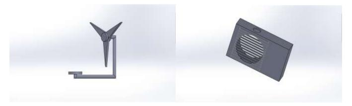
The turbine will be a conventional 3 blade horizontal axis wind turbine attached right behind the fan of the outdoor unit of the air compressor leaving a gap of 100mm in between the actual compressor and the wind turbine this will lead to a better wind flow and optimal use of space. The turbine will be mounted on the outdoor unit with the help of connecting rods, these rods will be responsible to support the turbine with the help of the outdoor unit.
