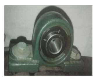
Fig- 8: Pedestal Bearing
