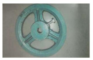
Fig- 6: Large Pulley
