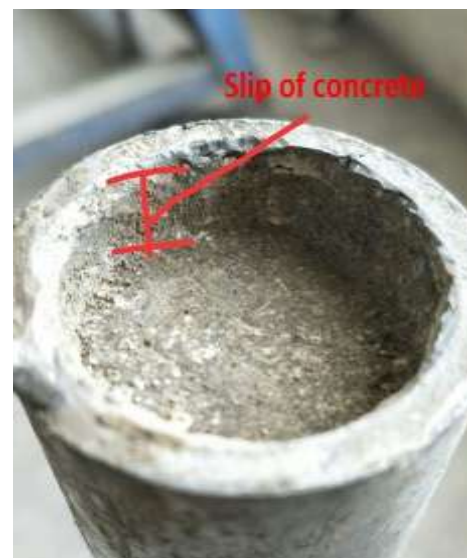
Fig -4: SCCFST column specimen after push-out test
