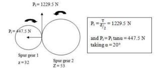
Fig- 7: Force analysis of Spur gears
