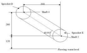
Fig-14: Drive from shaft 4 to shaft 5
