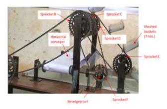
Fig-4: Drive from sprocket A to the conveyors through chain drives and bevel gear drive.
