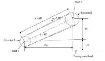
Fig-13: Drive from shaft 3 to shaft 4
