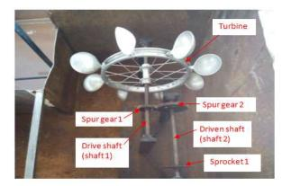
Fig-1: Turbine coupled with spur gear drive
