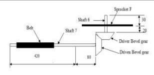
Fig-16: Bevel gear drive
