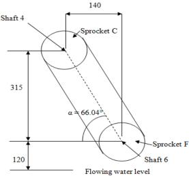
**Fig-15:** Drive from shaft 4 to shaft 6
